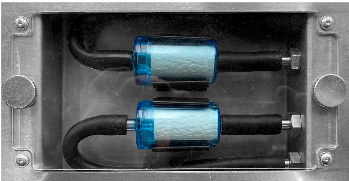
3.4 Filter for zero air for rinsing & generation of ions in the diffusion charger (top view)
